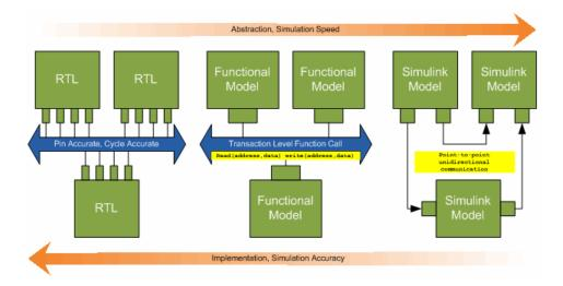
The functional model provides a sort of halfway point between the speed you can achieve with abstraction and the accuracy you get with implementation.
